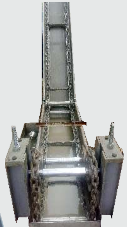
Submerged Ash Conveyor
